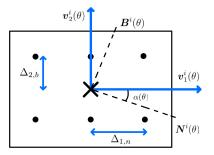
$\alpha$  is parametrized by another Fourier series, giving the coil the freedom to twist in space.
